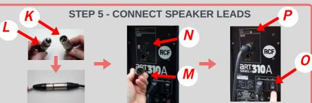
Connect speaker leads from the S-MIX (K) to the supplied extension lead (L). Connect the other end (M) to the back of the speaker (N). Switch on the speakers (O). The "I" on the switch should be pressed in & the Yellow "Power On" LED Indicator should be lit (P). Ensure the volume control is set to FULL volume on both Speakers (Q)
