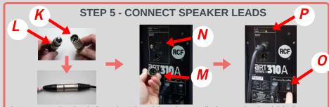
Connect speaker leads from the Mixer (K) to the supplied extension lead (L). Connect the other end (M) to the back of the speaker (N). Switch on the speakers (O). The "I" on the switch should be pressed in & the Yellow "Power On" LED Indicator should be lit (P). Ensure the volume control is set to FULL volume on both Speakers (Q)
