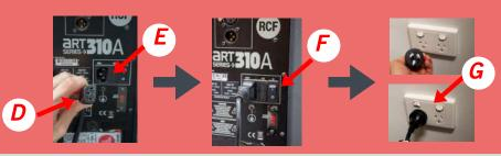
Plug the power lead (D) into the back of the speaker (E). The power lead is located in the top area of the speaker bag. Ensure power switch is turned OFF (F)
